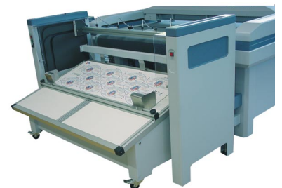
Automatic feeding systems for sheets (or from roll) available
