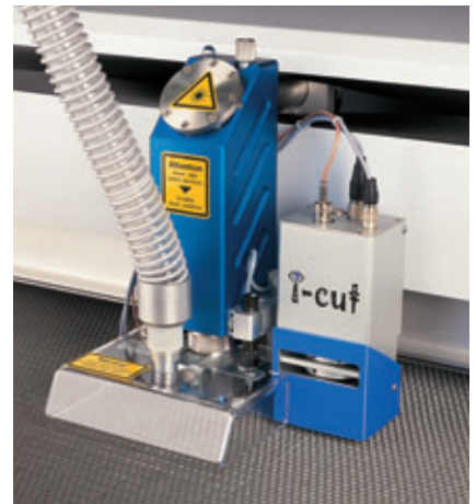
Material support to work with veneer or plastic foils. Camera system adapted.
